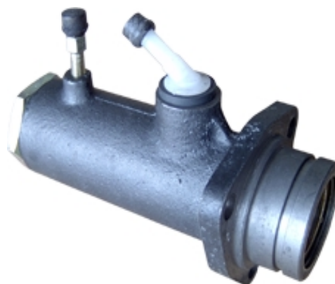
Glavni cilindar 1468112, \phi 38,1, TAM 1001, 75, 60, 80T3, T5, A5, A6, 110, T10, 125, T10K, 125T10G, 260, A116m, A116P, A120T, 120L, vilj. INDOS, D2,5t, vilj.Pobeda T.U.50
